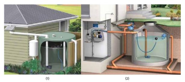
Figure 3.2 Catchment Ponds (1) on the ground and (2) underground (Source: Stormsaver 2017)
